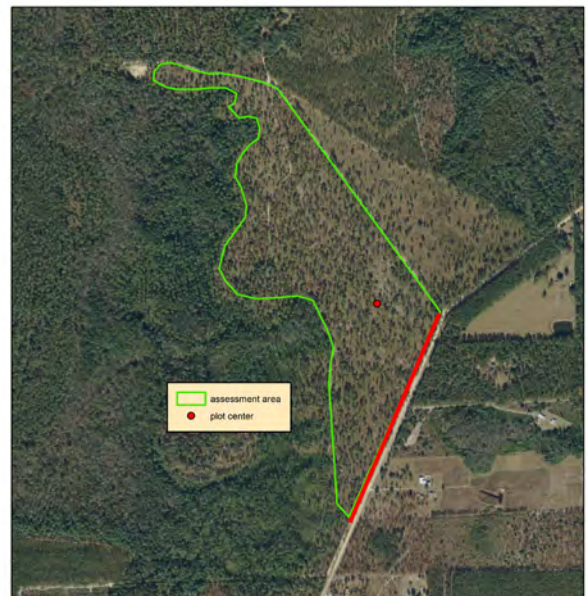
Figure 7. An assessment area with the perimeter bordered by natural area depicted in green and the perimeter bordered by non-natural area depicted in red. Perimeter measurements are easily calculated in GIS.
